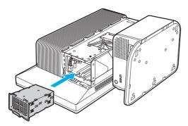
13 Replace the hard disk cover and the back panel, and then place the computer upright.
